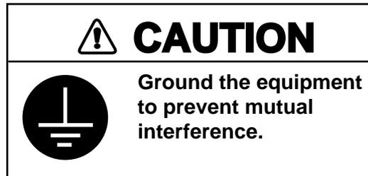
**Note:** Use a “closed” lug to make the ground connection at the display unit. Do not use an “open-type” lug (
